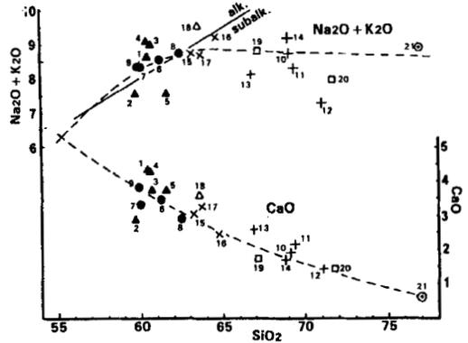
Fig. 4. Na<sub>2</sub>O + K<sub>2</sub>O and CaO vs. SiO<sub>2</sub> diagram, in weight percent. Alkali-subalkali division: Irvine & Baragar (1971). The alkali-lime index is roughly estimated between 56 and 47. Same nos. and symbols as Fig. 2.
