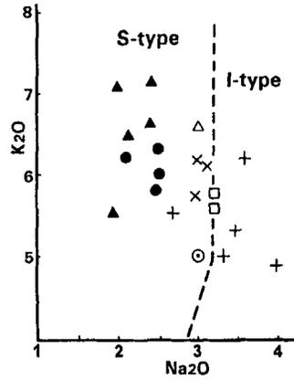
Fig. 6.  $\text{K}_2\text{O}$ - $\text{Na}_2\text{O}$  diagram, in weight percent. The S- and I-type division: White & Chappel (1977).
