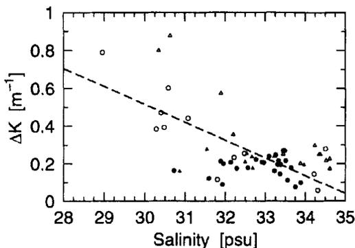
Fig. 9. Calculated values of  $\Delta K$  as a function of salinity  $S$  for the 38 optical stations where  $S$  was available. Explanation:  $\circ$  = Greenland Sea, 1991;  $\bullet$  = northern Barents Sea, 1991;  $\triangle$  = Greenland Sea, 1993;  $\blacktriangle$  = northern Barents Sea, 1993. The dashed line is the best fit to the observations from the Greenland Sea in 1991.
