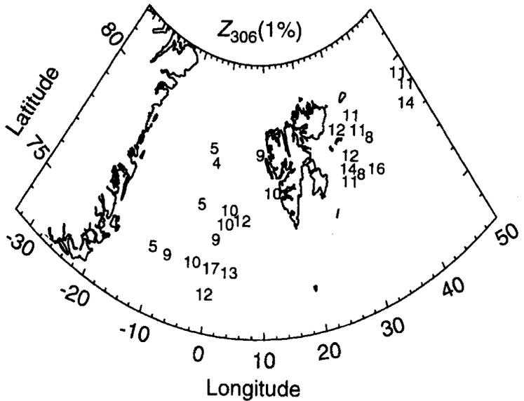
Fig. 6. Distribution in August 1991 and 1993 of the depths  $Z_{306}(1\%)$  where the downward UV-B irradiance is reduced to 1% of its surface value.
