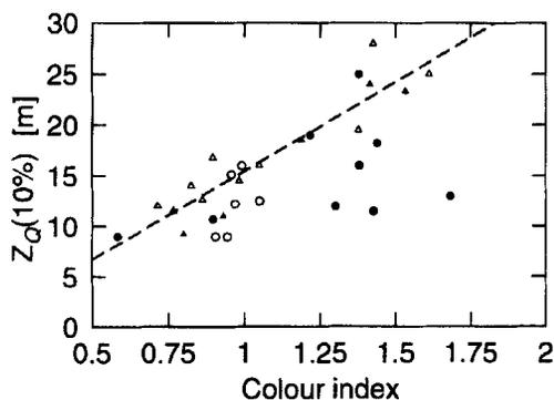
Fig. 10. The 10% depth of integrated quanta irradiance,  $Z_{\alpha}(10\%)$ , as a function of the colour index at 0 m (symbols as in Fig. 9). The dashed line gives the best fit to the observations from 1993.
