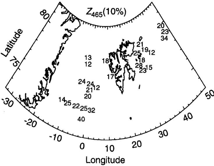
Fig. 7. Distribution in August 1991 and 1993 of the 10% depth for downward blue irradiance,  $Z_{465}(10\%)$ .
