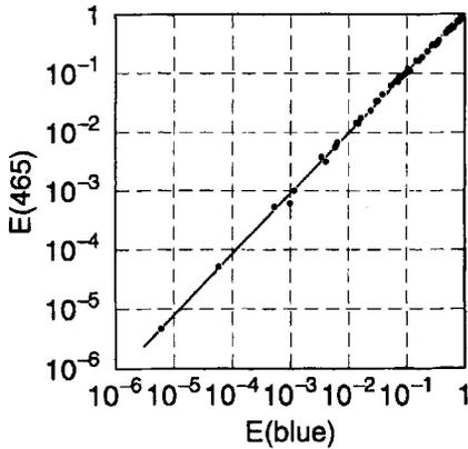
Fig. 1. Narrow band irradiance  $E(465)$  at 465 nm as a function of the broad band irradiance  $E(\text{blue})$  recorded with Schott filter BG12 + GG5, based on eight optical stations from the Norwegian Sea between the surface and a depth of 50 m. Both irradiances are normalised against their surface values (Aas & Berge 1976).
