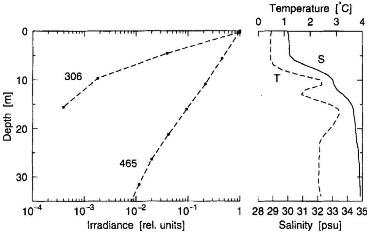
Fig. 3. Downward irradiances at 306 nm (corrected) and 465 nm, and temperature *T* and salinity *S* as functions of depth at the same station as in Fig. 2.
