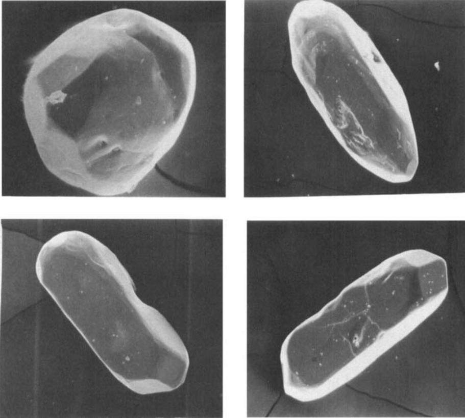
Fig. 2. Morphotypes of the zircon grains, scanning electro-micrographs. Upper left, morphotype 1,  $\times 480$ , upper right, morphotype 1  $\times 168$ ; lower left and lower right morphotype 2, both  $\times 240$ .
