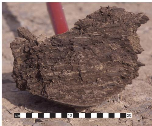
Fig. 8. Silty regolith sampled in the active layer 0.4 km east of the dyke. Shaly structure from the parent rock is well preserved.
