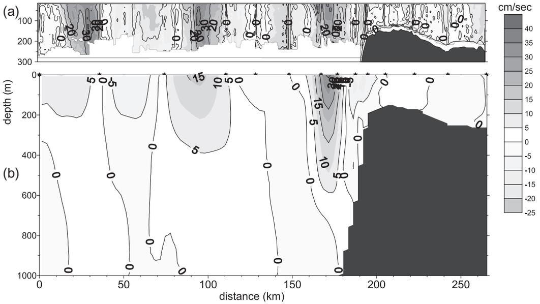
Fig. 4. (a) Vertical distributions of the perpendicular component of ADCP measured current, and (b) calculated baroclinic geostrophic current with reference level 1000 m at transect S.
