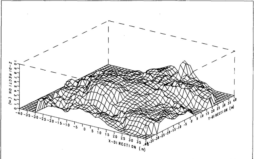
Fig. 5. Typical bottom topography features of multi-year ice as mapped with a scanning sonar at 78.8°N and 29.7°E September 1989. The dimensions of the box are 40 m × 40 m × 10 m. The flat areas in the corners are areas with no data due to ship or ridge shadows. The grid spacing is 2 m.
