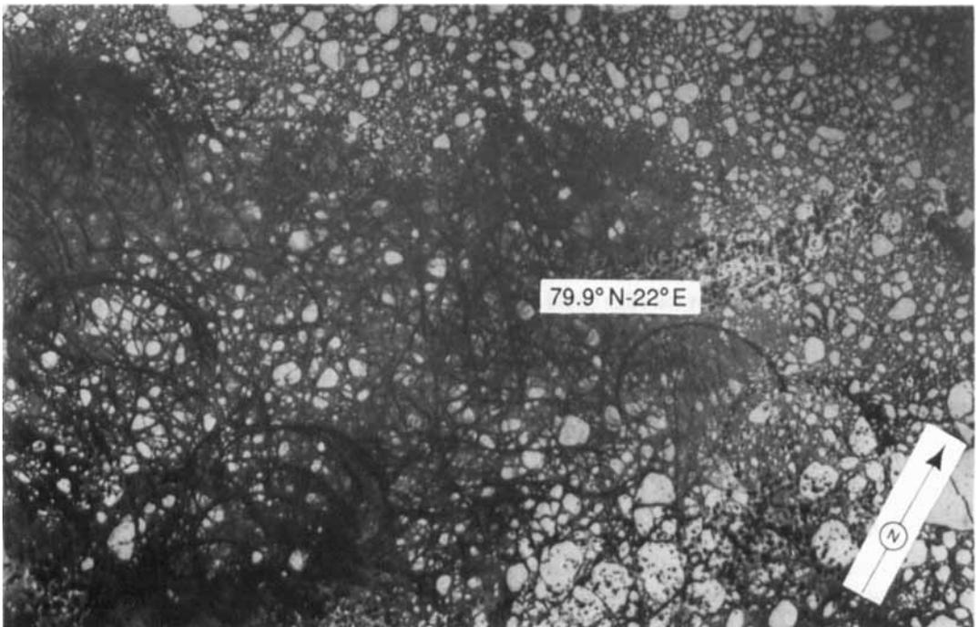
Fig. 6. Trails after grounded icebergs on Spitsbergenbanken caused by tidal or inertial effects in the moving ice field. Landsat TM image 1 June, 1988. The loop diameter is about 15 km.
