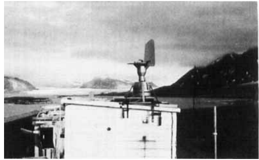
Fig. 2. The Burkard pollen and spore trap on the roof of the research station in Ny-Ålesund. Photo: S. Johansen 1986.
