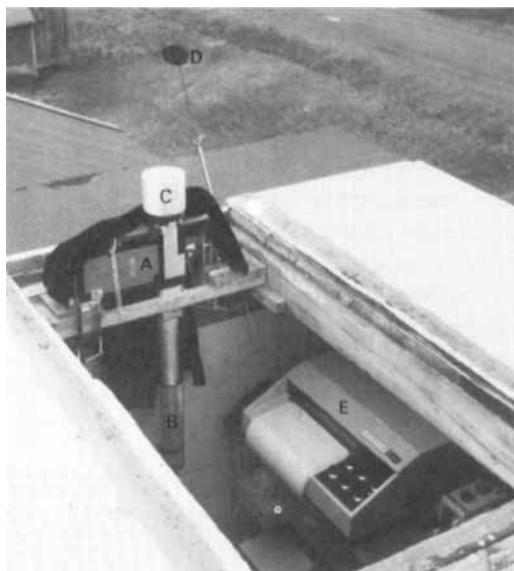
Fig. 1. Monochromator and additional equipment mounted on the observation platform. A: monochromator, B: photomultiplier, C: integrating sphere, D: sun screen, E: recorder.
