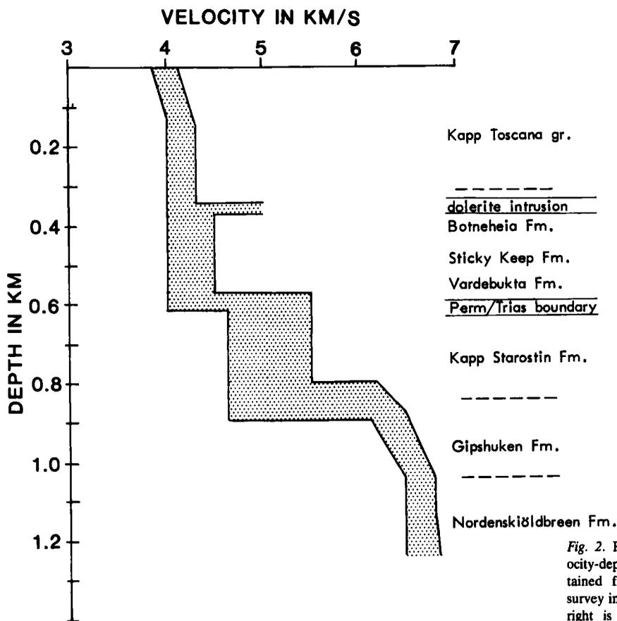
Fig. 2. Range of possible velocity-depth distributions obtained from the land-seismic survey in Agardhdalen. To the right is the geological interpretation of the velocity model.
