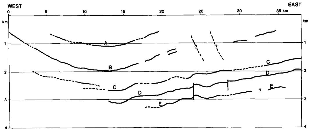
Fig. 5. Depth-converted geoseismic section along van Mijenfjorden from west to east (A-A' in Fig. 1). The following ages of reflectors are suggested: A. near base Tertiary; B. within early Cretaceous, possibly the Festningen Member; C. near top Triassic or in the middle of Triassic; D. a sill in the middle Triassic or at the Triassic/Permian boundary; E. the Triassic/Permian boundary or near the top of the Gipsdalen Group (early Permian).
