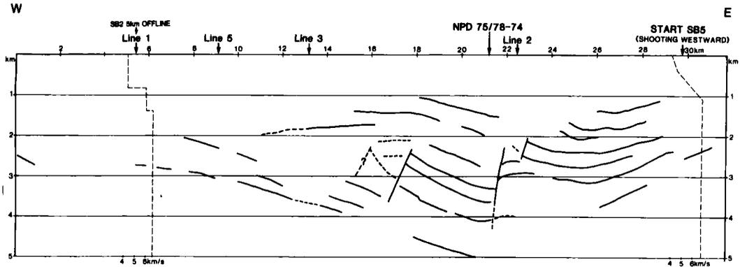
Fig. 6. Depth-converted geoseismic section across the fault zone in northern Storfjorden from west to east (B-B' in Fig. 1). Velocity-depth solutions of adjacent sonobuoy measurements projected onto line (locations in Fig. 1).
