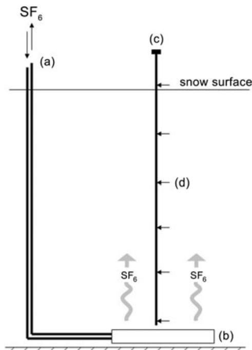
**Fig. 1** Schematic overview of the gas diffusion technique. The trace gas, SF<sub>6</sub>, is circulated by a pump (a) down to the air-permeable membrane (b), which allows the trace gas to diffuse out into the surrounding snow. Air samples were withdrawn with a syringe through 1.6-mm diameter tubing attached to an avalanche probe (c), thereby allowing the sampling of air (d) at distinct levels.
