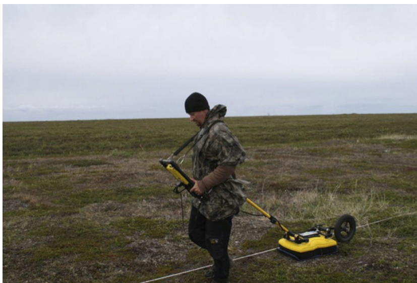
Fig. 4 The site presented a flat surface free of obstructions, making the deployment of geophysical instruments very easy. Shown here, Thomas Urban with Noggin ground-penetrating radar system. (Photo by Christopher Wolff.)
