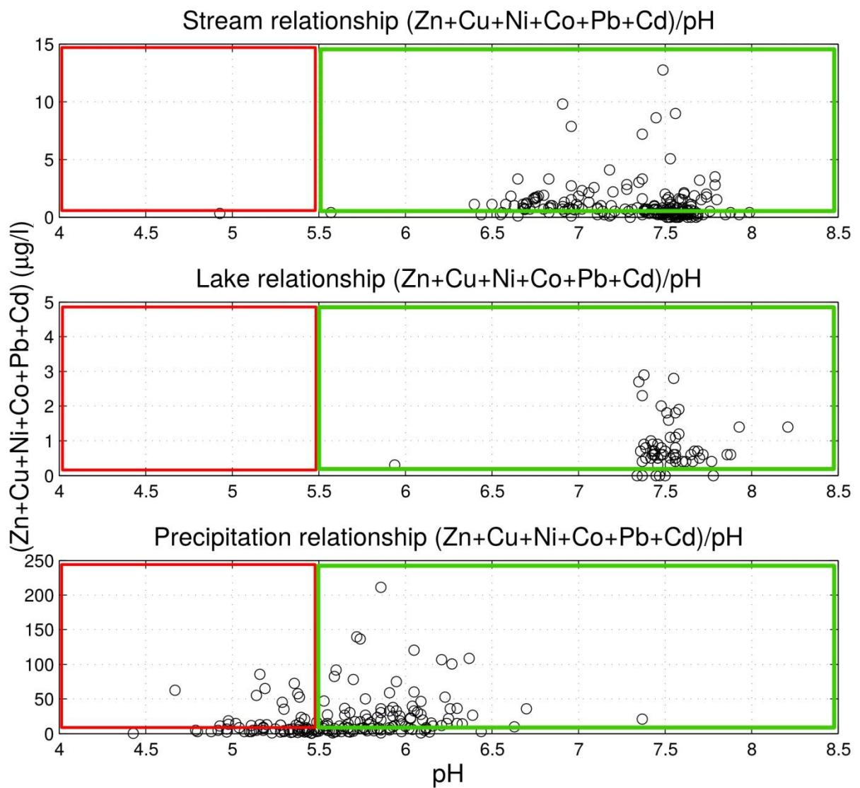
**Supplementary Fig. S4.** The relationship between metal concentration and pH in the surface waters and atmospheric precipitation.
