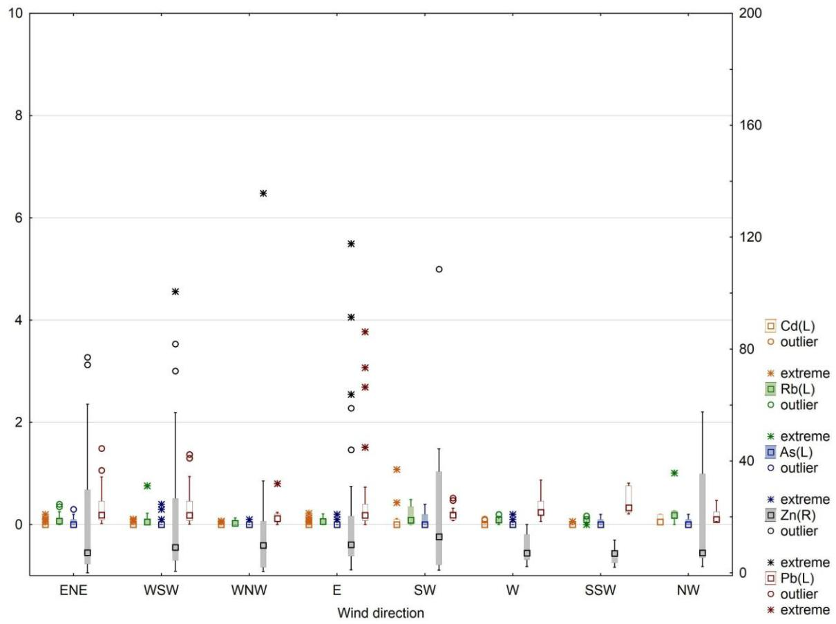
**Supplementary Fig. S3.** Box and whisker plot of the concentrations of the five variables in the discriminant analysis model based on wind direction classification, marking all quartiles and the extent of non-outliers. Please note that Zn concentrations are plotted on the right Y axis.
