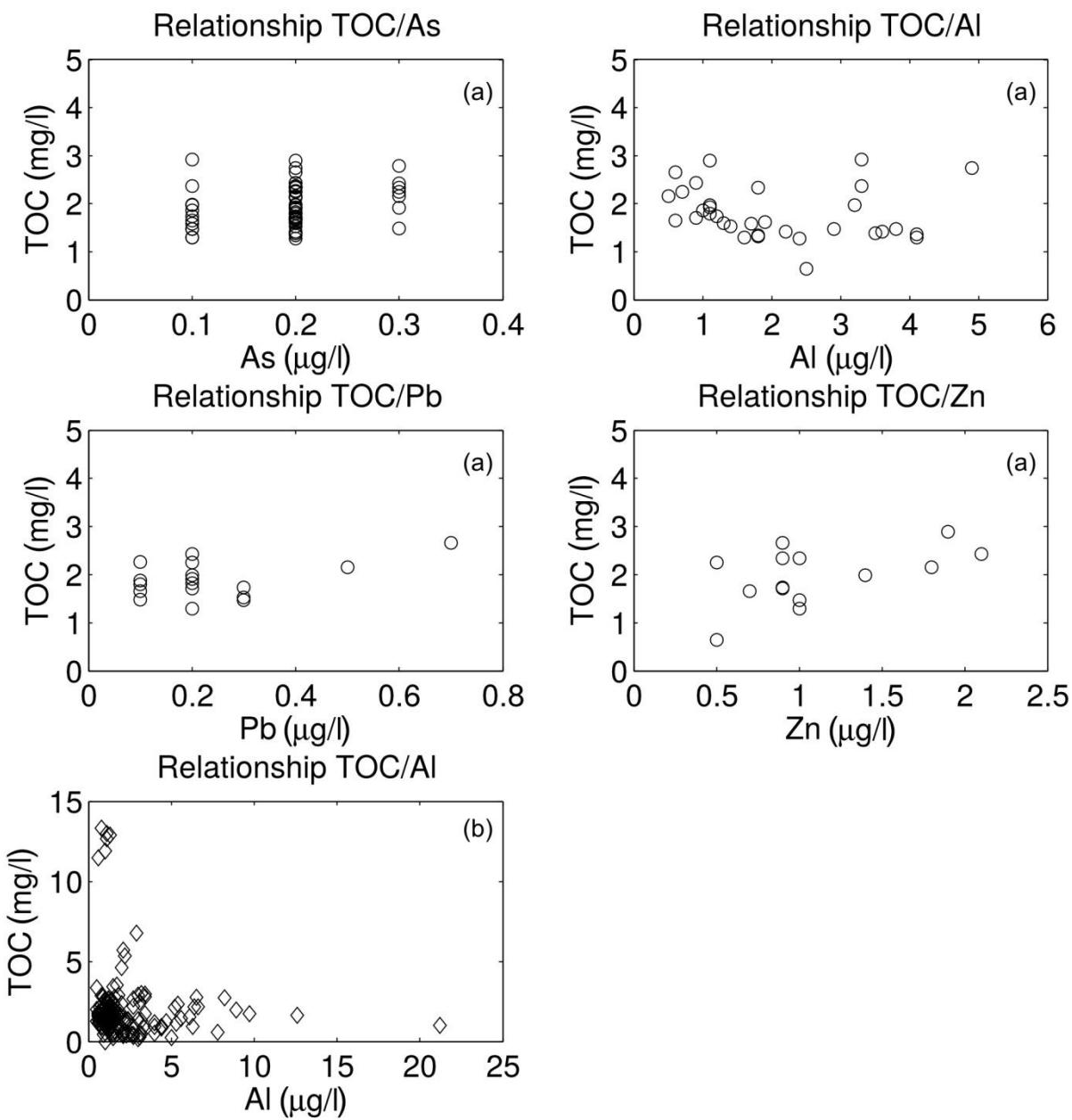
**Supplementary Fig. S5.** The occurrence of relationships between chosen elements and the total organic carbon (TOC) in the samples collected from (a) the Fuglebekken lake and (b) the Fuglebekken stream.
