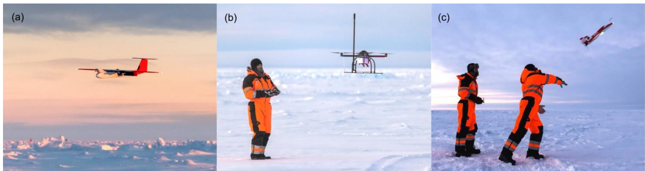
Supplementary Fig. S1 (a) The meteorological mini aerial vehicle in flight above the sea ice, (b) the quadcopter landing procedure and (c) launch of the small unmanned meteorological observer for a mission.
