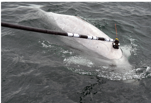
Fig. 2 DTAG deployment on a sub-adult beluga, using a handheld carbon fibre pole, within 1 m of the blowhole.
