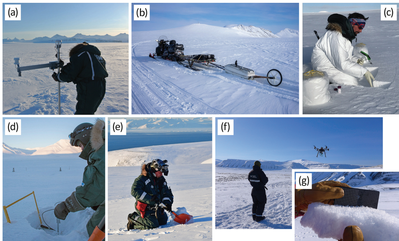
Fig. 3 Snow science in action: (a) setting up an automated ultrasonic snow surface height sensor; (b) ground penetrating radar survey of snow thickness and stratigraphy; (c) collecting surface snow samples to measure concentrations of black carbon aerosols; (d) measurements of several snow parameters along transects covering different ecological gradients to validate snow models; (e) measurements of snow depth and basal ice thickness; (f) operation of ground penetrating radar on a drone; (g) measurement of snow grain size. (Photos: a–c, Jean-Charles Gallet, Norwegian Polar Institute; d–e, Ketil Isaksen, Norwegian Meteorological Institute; f–g, Hannah Vickers, NORCE Norwegian Research Centre.)
